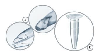
Tests at  $30,000 \times g$  show that other microcentrifuge tubes (a) might burst during centrifugation resulting in sample loss - Eppendorf Safe-Lock Tubes (b) allow fast and safe centrifugation of your samples\*1!
